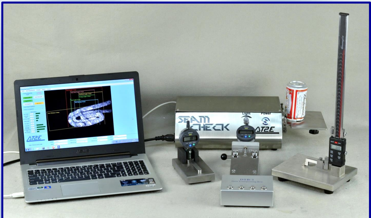
SeamCheck connecting with optional gauges through DTB-1
