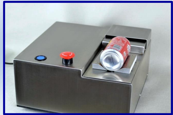
Optional seaming cutting saw: ANSS & SS-1
